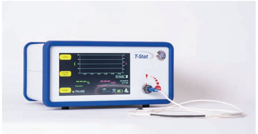
T-Stat 2.0 monitor using the 2.5cm surface sensor
